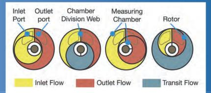
The flow of the chemical causes the rotor to rotate. Each rotation produces one pulse.
